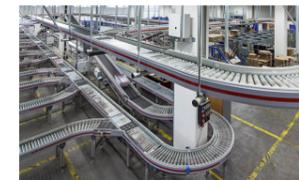
Conveyor system transports bins containing items retrieved from automated warehouses to the picking area.
