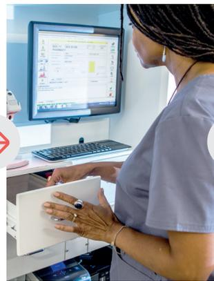
**3** · BoxPicker retrieves the appropriate medication box based on space availability and delivers the box to an access drawer at the operator station.
