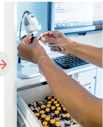
**4** · Once the box has been delivered, the technician opens the access drawer, scans the medication to be loaded and places it in the assigned location.
