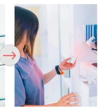
1 · A technician logs into the operator station and selects an order received through an interface with the hospital's information system and/or ADC<sup>1</sup> vendor 2 · BoxPicker picks only the correct medication box and places it in an access drawer at the operator stationdate 3 · Once the box has arrived, a green light indicates the drawer is unlocked and can be opened
