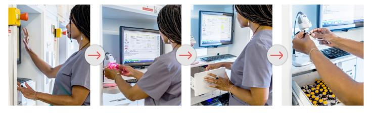
A technician logs into the BoxPicker operator station and selects the «Load» option 2 · A technician scans the medication to be loaded and enters the quantity and expiration date 3 · BoxPicker retrieves the appropriate medication box based on space availability and delivers the box to an access drawer at the operator station 4 • Once the box has been delivered, the technician opens the access drawer, scans the medication to be loaded and places it in the assigned location
